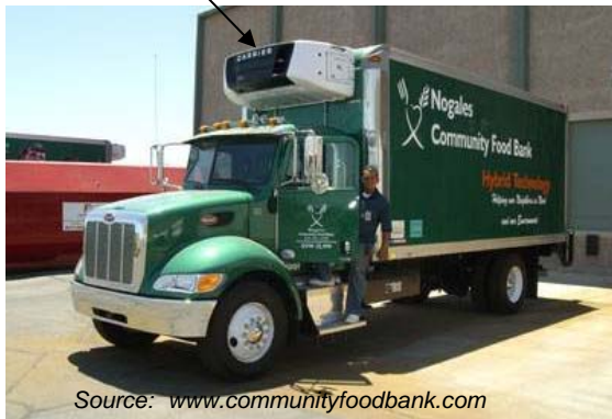
Refrigeration: > 20kW, 3-phase
