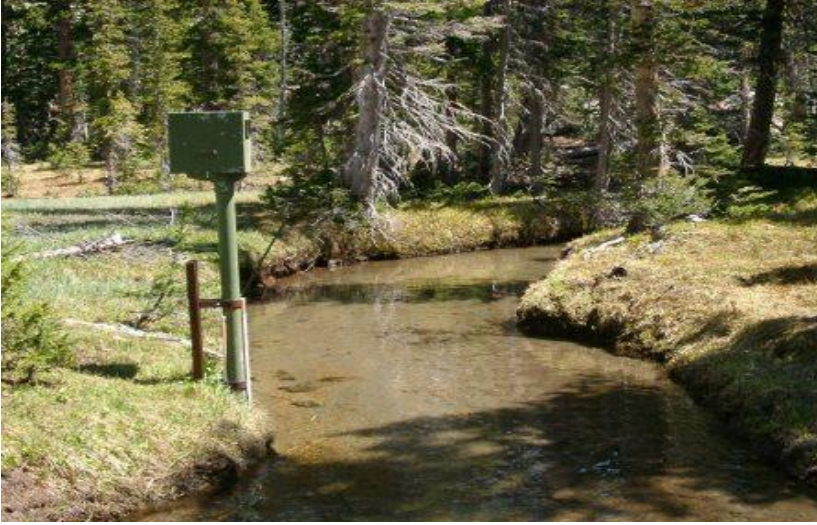
Figure 26: Stream Gauge on Andrews Creek, CO;
