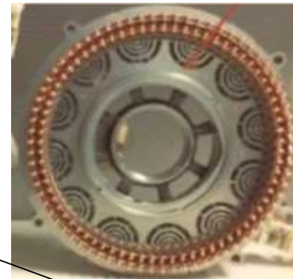
Generator (ferrite) Top eff: 94%
