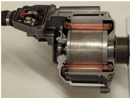
GM induction starter-generator
